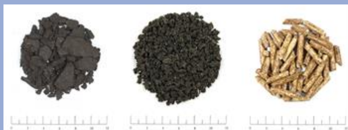
Granulated lignite (left) sewage sludge (middle), pelletized low grade wood (right)
