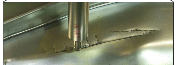
incremental sheet metal forming at IWU
