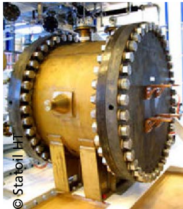
30 bar AEL stack in pressure compartment
