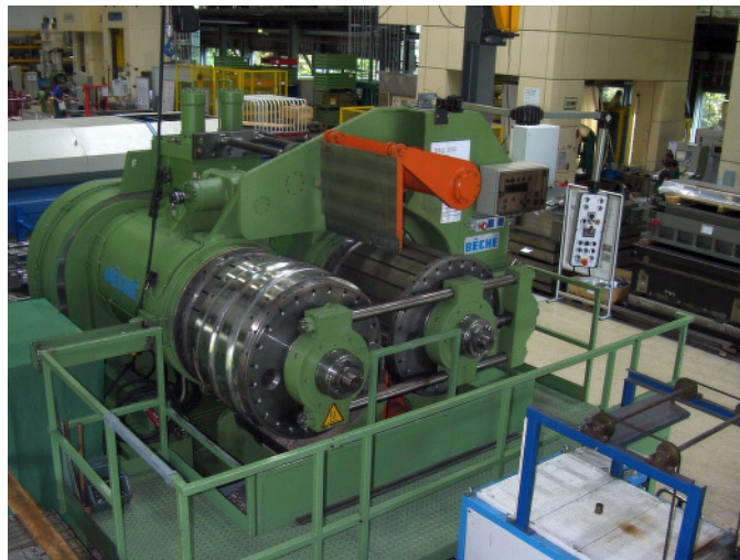
Fig. 1: Round tool rolling machine RBQ 1000 in the workshop of Fraunhofer Institute
