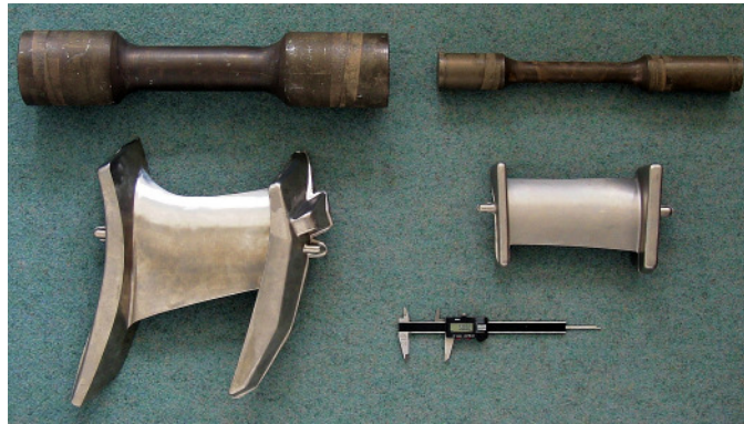
Fig. 3: Additional examples of cross rolled preforms of aero engine vanes
