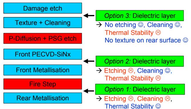
Fig. 1. Formation of a dielectric layer within an industrial solar cell process.
