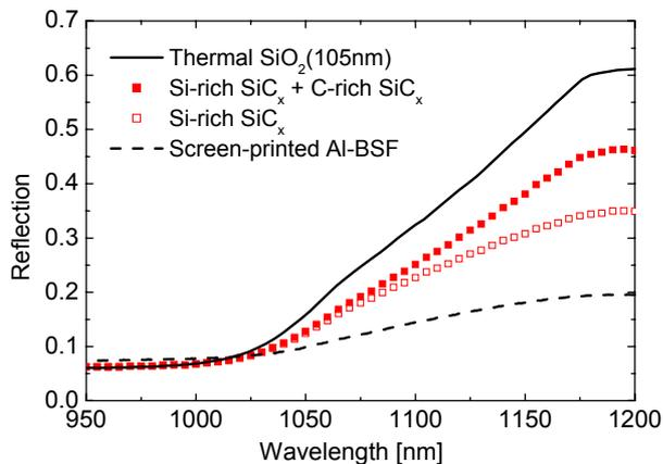
Fig. 4 Reflection of solar cells with different rear surface structures.
