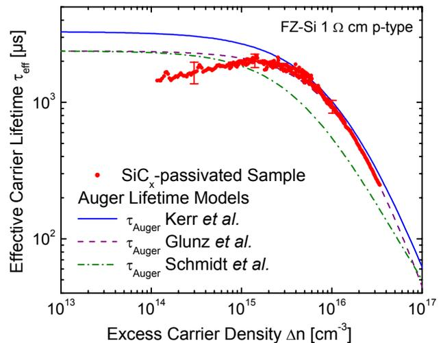
Fig. 3. Effective lifetimes of a 4" 1 Ω cm FZ-Si wafer passivated with SiC<sub>x</sub> and three recent Auger lifetime models (Kerr *et al.* [16], Glunz *et al.* [17] and Schmidt *et al.* [18]).
