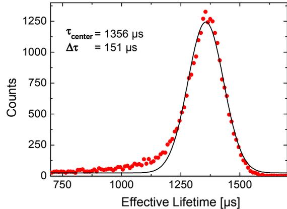
Fig. 2. Spatial lifetime distribution on a 4" 1 Ω cm FZ wafer passivated with an optimized SiC<sub>x</sub> layer after an in-situ plasma cleaning step.
