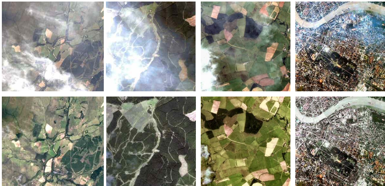
Figure 1: Example of a haze reduction in IKONOS-images (upper row: images with haze, lower row: corrected images); Source: www.atcor.de (IKONOS-Data: Courtesy of European Space Imaging / © European Space Imaging GmbH)
