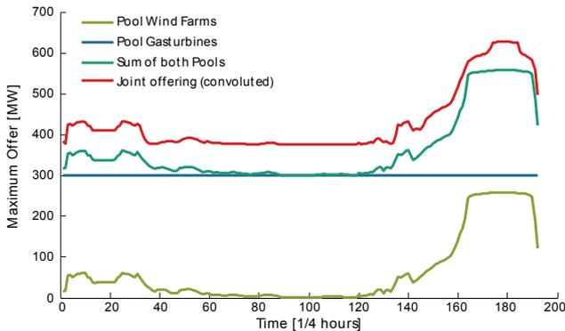
Figure 1. Pooling of a day-head forecast of wind farms of 1 GW and a 1 GW pool of five gas turbines in total
