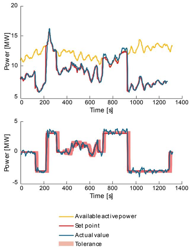
Figure 6. Field test results for one wind farm
