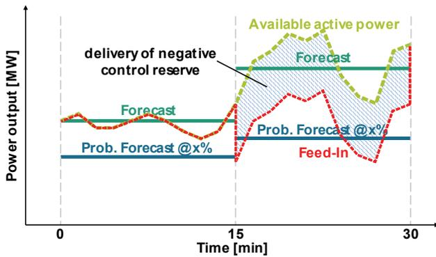
Figure 5. Proof of control reserve under the mechanism "available active power"
