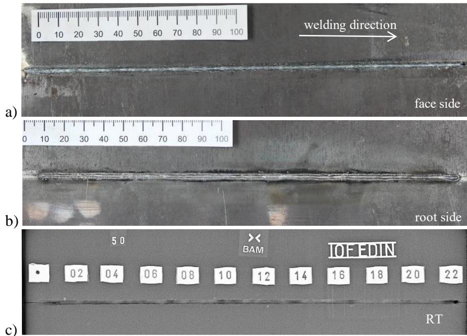
Figure 2 Photographs of (a) face side, (b) root side, (c) RT film of autogenous laser welded joint produced using 18 kW laser power, 2 m/min welding speed and 25 l/min argon shielding.
