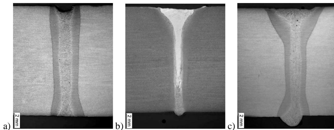
Figure 5 Macrographs of cross sections taken from (a) autogenous laser welded joint, (b) HLAW joint produced using filler wire ENiCrMo-3 and (c) HLAW joint produced using filler wire Bohler Tht 11TT
