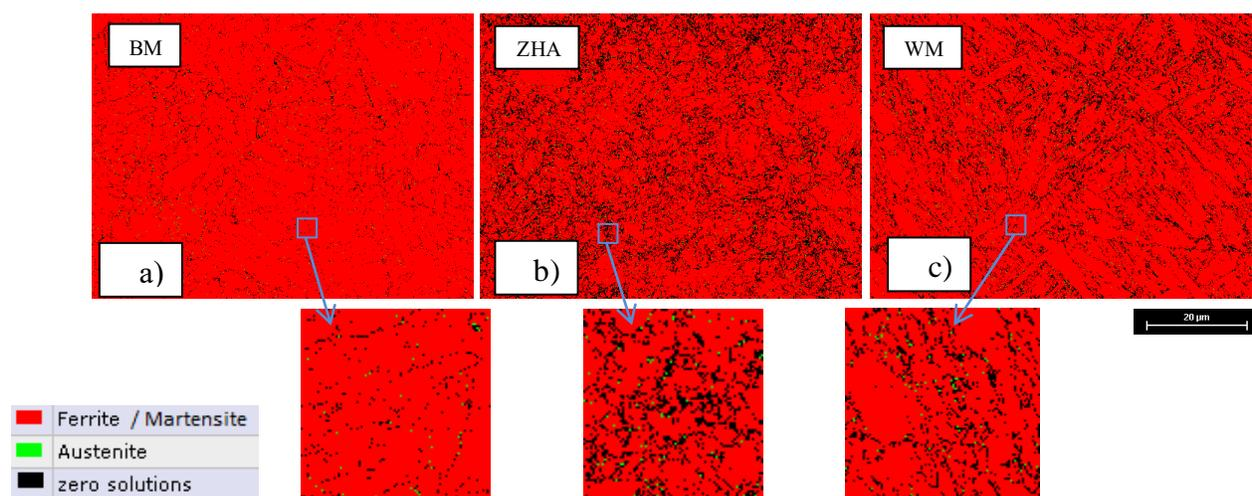
Figure 7 EBSD phase maps showing phase composition of the base metal (a), laser weld HAZ (b) and laser WM (c)
