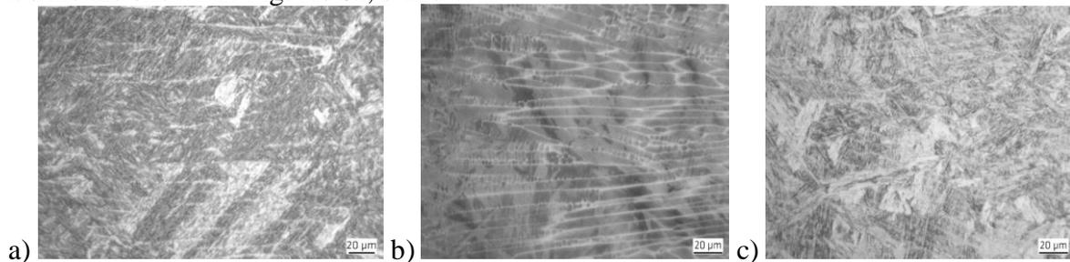
Figure 6 Optical micrographs of weld metal for (a) autogenous laser welded joint, (b) HLAW joint produced using filler wire ENiCrMo-3 and (c) HLAW joint produced using filler wire Bohler Tht 11TT
