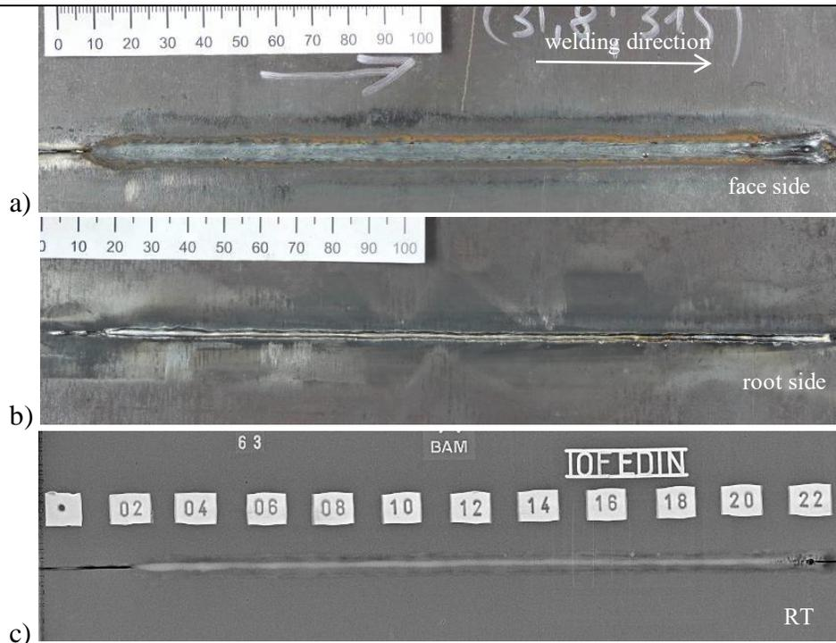
Figure 4 Photographs of (a) face side, (b) root side, (c) RT film of HLAW joint produced using 17 kW laser power, 2.8 m/min welding speed, 16 m/min wire feeding rate (Bohler Tht 11TT) and 25 l/min argon+18% CO<sub>2</sub> shielding.
