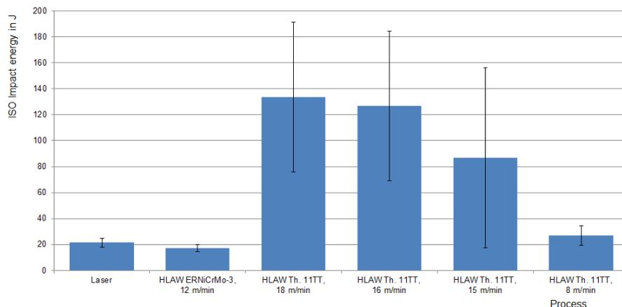
Figure 9 Impact absorbed energy at test temperature  $-196^{\circ}\text{C}$  for laser beam welds as well as HLAW welds made using different filler metals with different wire feeding speeds.
