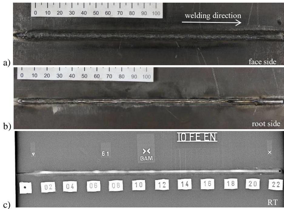
Figure 3 Photographs of (a) face side, (b) root side, (c) RT film of HLAW joint produced using 17.5 kW laser power, 2.6 m/min welding speed, 12 m/min wire feeding rate (ENiCrMo-3) and
