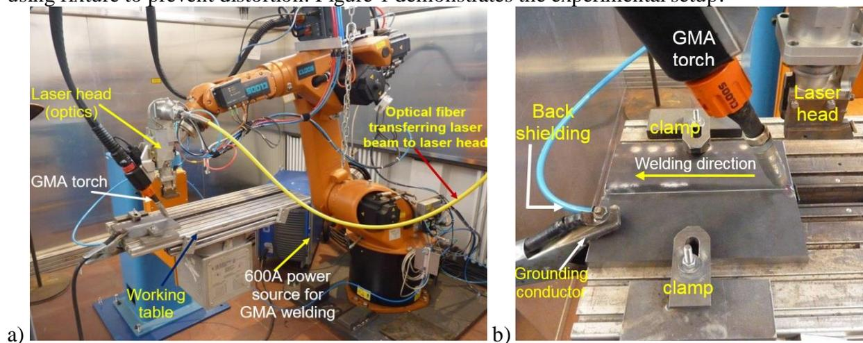
Figure 1 Laser and laser-GMA hybrid welding system used for experiments: (a) laser head and GMA torch are mounted on a 6-axis welding robot and (b) no gap square butt joint alignment, clamping and back shielding preparation
