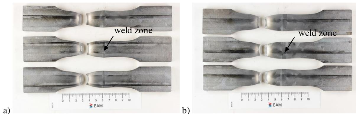
Figure 8 Example of tensile test fractured specimens of (a) laser beam welded joint, (b) HLAW welds
