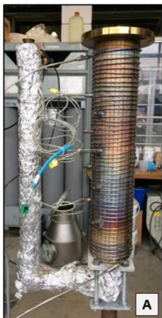
Figure 4: Reactor for catalytic vapour upgrade [19]
