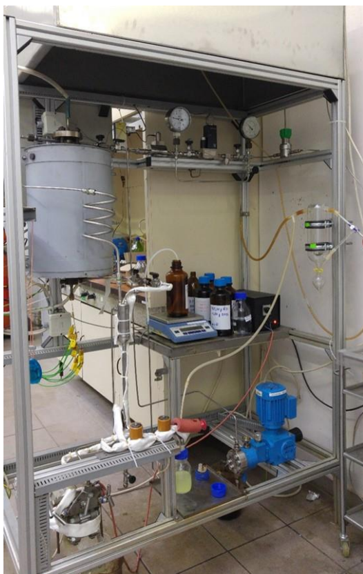
Figure 7: Continuously operated test rig for mild catalytic hydrotreatment
