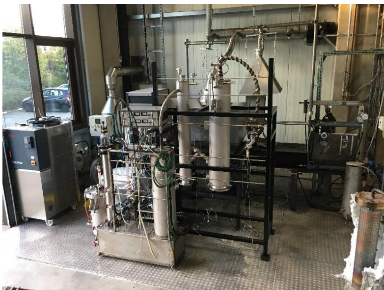
Figure 5: AFP plant with two stage condensation (original single stage condenser and ESP in front) [19]
