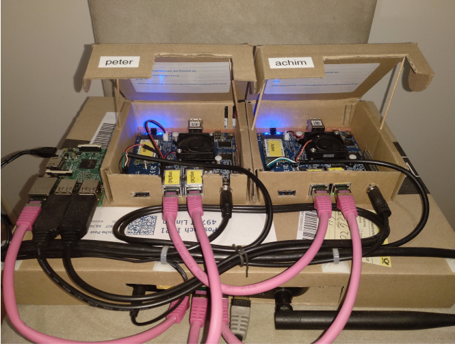
Fig. 3: The hardware setup of our test-bed: Two Minnow-Boards acting as Profinet peers are connected directly via Ethernet. A Raspberry Pi 3B+ is acting as a control node. Management traffic is routed through dedicated ports; RS232 terminals are in service as backup. The left MinnowBoard is our chosen Profinet controller while the right board is our Profinet device.
