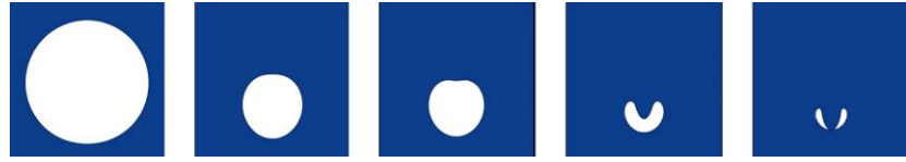
Figure 4. Typical cavitation bubble collapse simplified model simulations.
