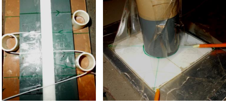
Figure 6. Example of experimental set-up to measure detonation velocity (left) and pressure (right).
