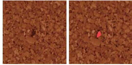
Figure 2: Image of cork tile (left), detected defect (right)
