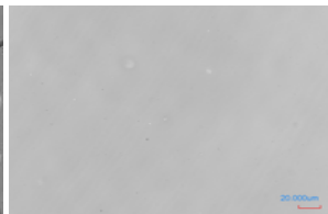
Figure 2: Smooth whey coating with plasticizer (100 Sorbitol)
