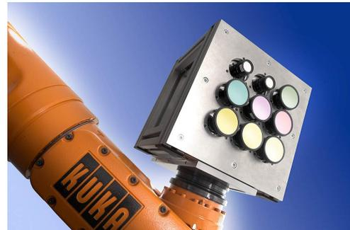
Figure 1. The camera array in combination with an industrial robot.
