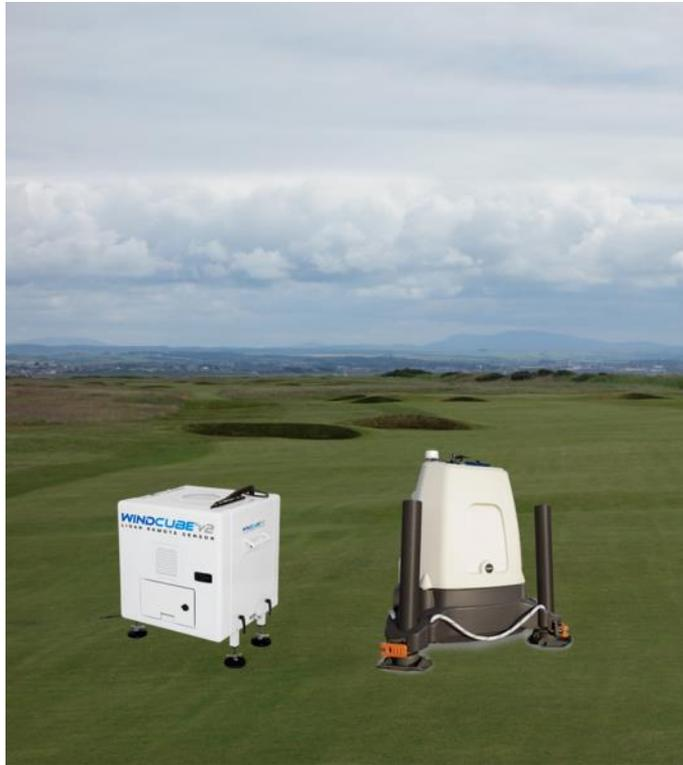
**Figure 1.1: Two wind lidars: pulsed lidar and continuous wave (CW) (©ZephIR/Leosphere) [21].**
