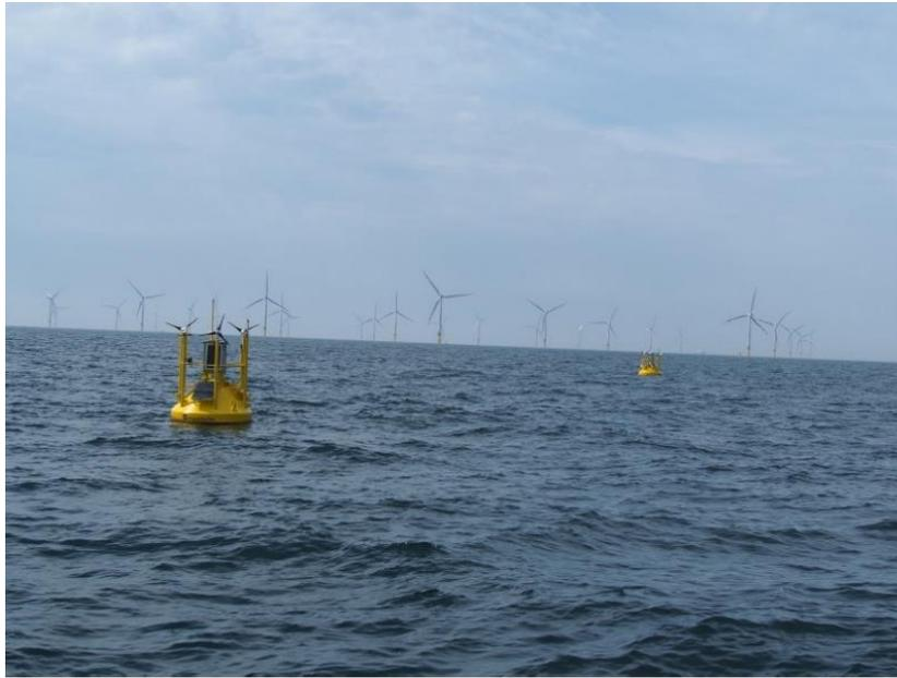
**Figure 1.3: Fraunhofer IWES wind lidar buoy [2]. The lidar is adapted to a common marine buoy and protected from salt and water through an aluminum box with special glass at the top so that the light beams are not distorted.**
