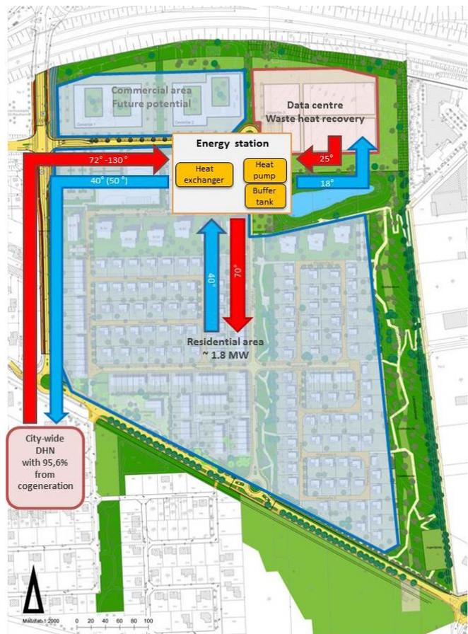
Figure 82. Excess heat recovery from data centre in Braunschweig/Germany.
