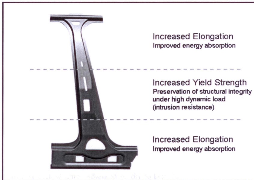
Fig. 2: B-pillar - optimized component properties for improved crash performance
