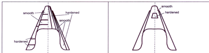
Fig. 13: Possible local structural improvements, hardening of tracks (left) and zones (right)
