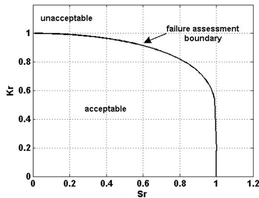
Figure 1: Failure Assessment Diagram (FAD)<sup>[5, 6]</sup> (strip yield model). Failure occurs when the calculated assessment point ( $S_r$ ,  $K_r$ ) reaches the failure assessment boundary. If the assessment point lies within the acceptable area the component is considered as safe.
