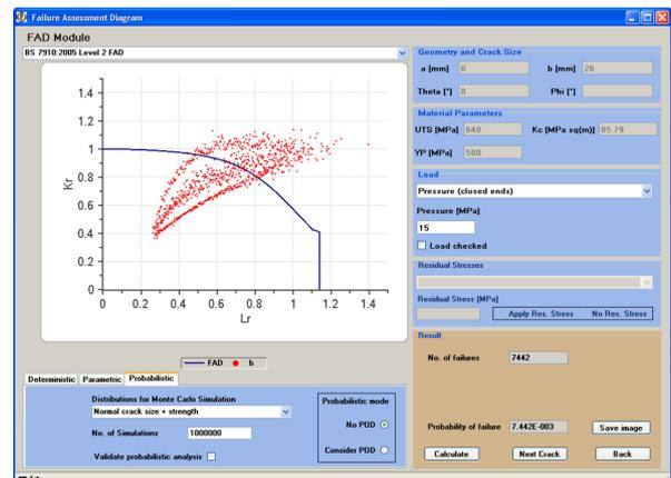
Figure 5: No NDT applied (assessment points for crack depth, red)
