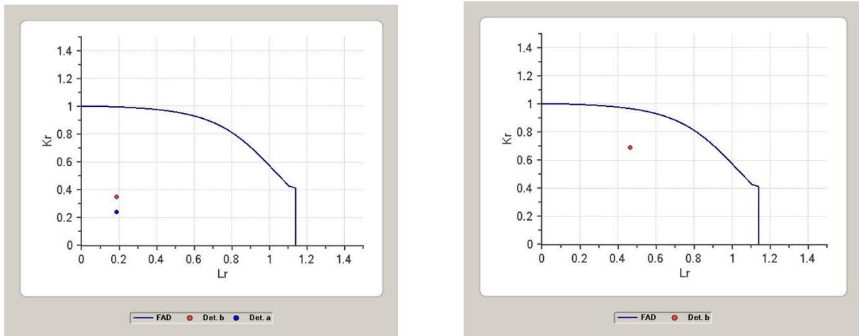
Figure 3: Deterministic FAD evaluation, Left: semi-elliptical crack (assessment point for crack depth, red and for crack width, blue), Right: circumferential crack (assessment point for crack depth, red)
