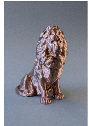
Polymer part via FDM, copper plated with PVD Source: Fraunhofer IST 2017
