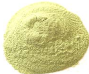
Material sample #3: Impregnated DuraForm PA12
