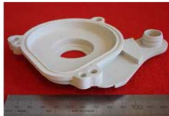
Material sample #2: PBT powder
