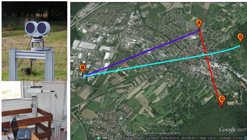
Figure 2. Left: boundary layer scintillometer BLS900 (top left: transmitter, bottom left: receiver). Right: aerial view of the paths of the three scintillometer measurements: purple line from the Fraunhofer IOSB (A, receiver) to the tower of the fire station (B, transmitter), red line from the Fraunhofer IOSB (A, receiver) to the Kreuzelberg (C, transmitter), and cyan from tower of the fire station (B, receiver) to the Bismarck Tower (D, transmitter). Map courtesy of Google Earth.
