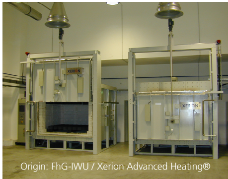
FIGURE 2: Electrical heated furnaces used for foaming
