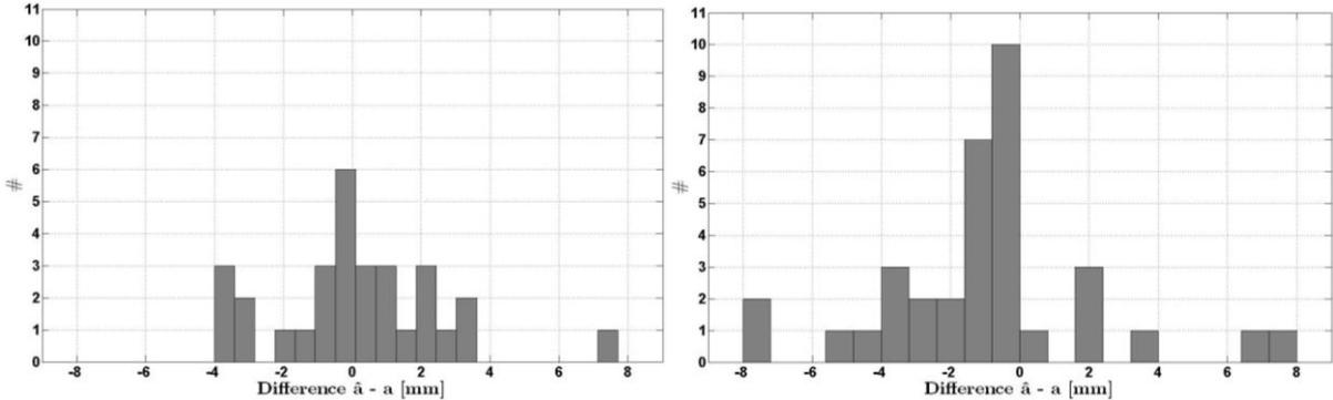
**Figure 8.** Differences between true flaw sizes and determined flaw sizes obtained from the measurements on the austenitic specimens. Left: RT phased array probe. Right: sampling phased array technique.
