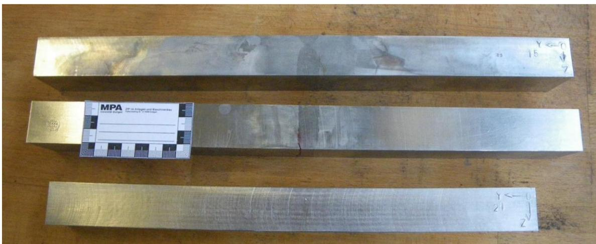
Figure 2. Austenitic test specimens with and without weld.
