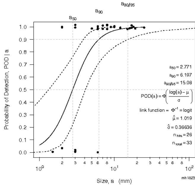
**Figure 5.** POD curve calculated from hit/miss data. For POD calculation the mh1823 software [14] was used.
