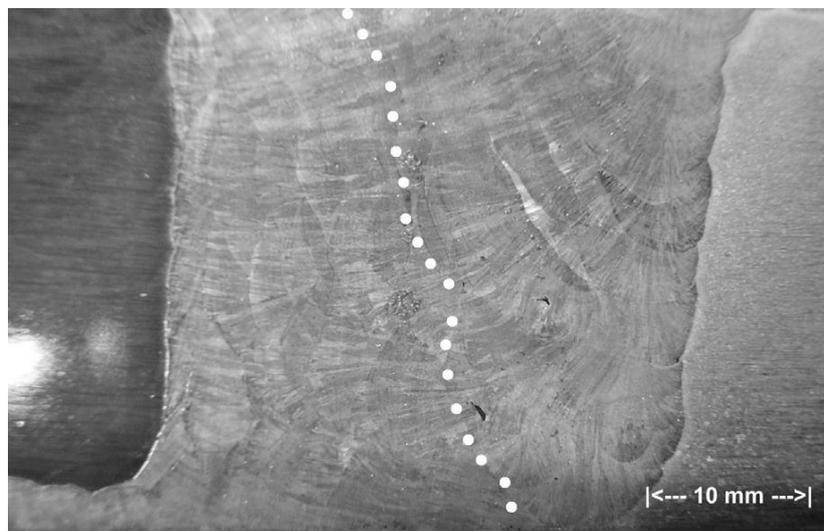
Figure 3. Cross section of the dissimilar weld.
