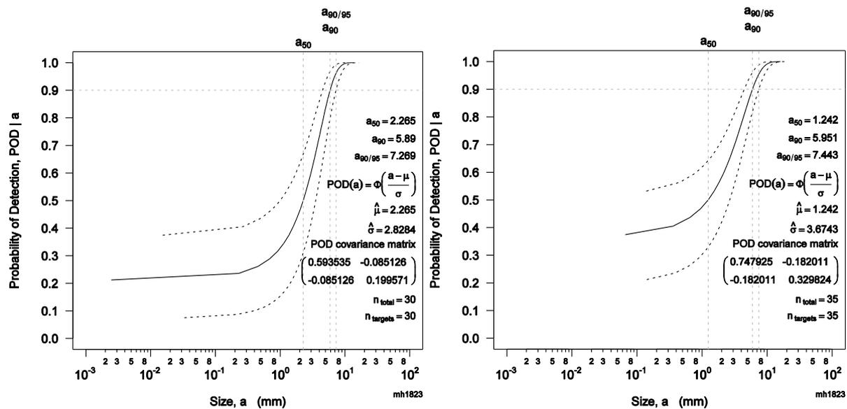
**Figure 9.** Left: POD curve from RT probe phased array data. Right: POD curve from SPA data. The POD calculation was carried out with the mh1823 software [14].
