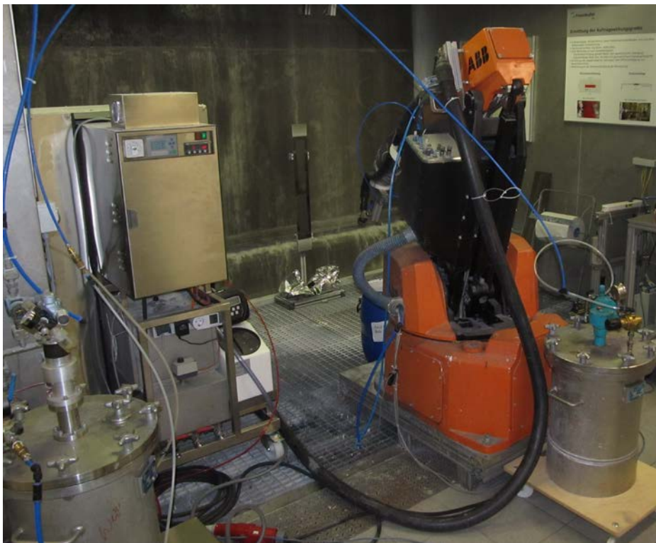
Fig. 1: Experimental setup with Krautzberger steam atomization in IPA-lab
