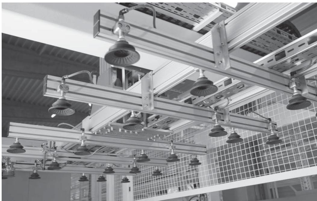
The vacuum gripper system can be used telescopically to both sides.
