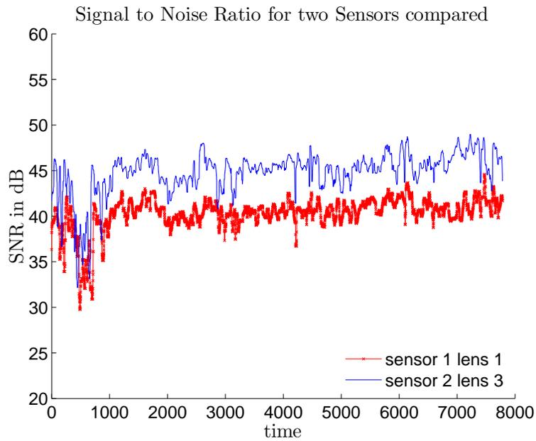
Figure 6. SNR results of the right lane for sensor 1 and sensor 2 equipped with the same lens for a long sequence of one measuring campaign (ca. 9min at 15 frames per second).
