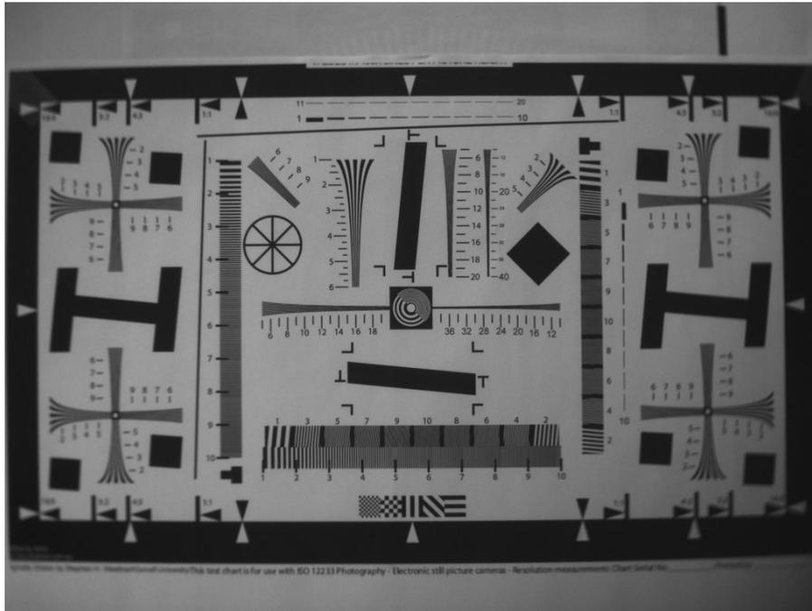
Figure 2. Example of one MTF measurement scene with ISO12233 target
