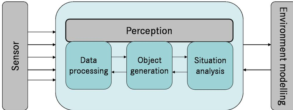
Figure 1. Structural layout of the perceptive components of a driver assistance system
