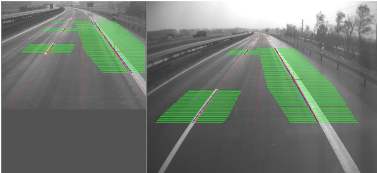
Figure 12. Lane feature extraction result with different lenses on wet road. Due to the different perspective, Sensor 1 with lens 5 (left) is capable of resolving features in the far distance, where sensor 2 with lens 6 fails to detect anything for the far part of the viewing area. This gain in distance for lens 5 comes with the loss of data in near distances, which are simply not covered by the field of view.
