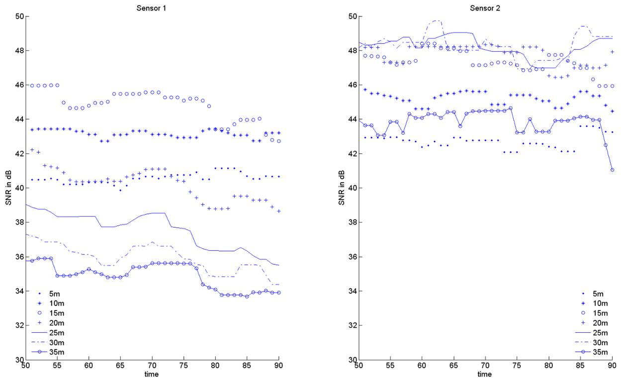
Figure 11. Comparison of the SNR evaluation for different distance segments of the sequence shown in Fig. 10. The low performance of sensor 1 with growing distance is represented by a low SNR for the segments above 30m. Sensor 2 shows superior performance for all segments. The bad quality of the road markings results in a moderate ratio for the near distance.
