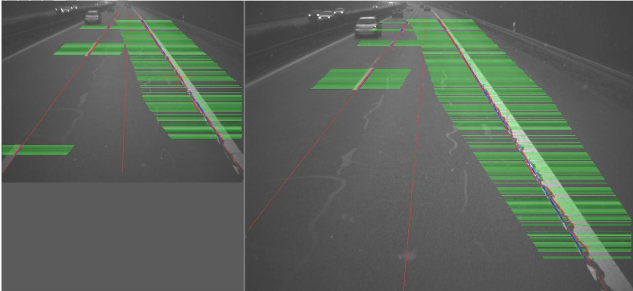
Figure 10. Lane feature extraction result for a dark scene with low marking quality. Green lines represent successful lane detections and the road model state is colored red. Sensor 1 with lens 1 on the left shows a significant performance loss against sensor 2 with lens 3 at far distance. In the near distance both sensors show incomplete detection of the lane due to bad quality of the markings.
