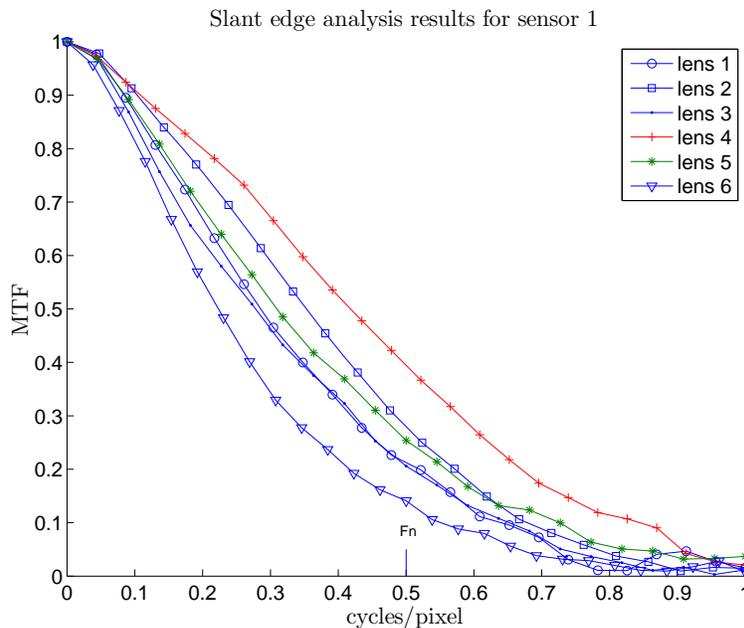
Figure 3. Normalised MTF for sensor 1 over cycles per pixel ( $F_n = \text{Nyquist Frequency}$ ). Lens 4 shows the best performance and lens 6 the lowest. The structurally identical lenses 1 and 3 show the expected equal performance.
