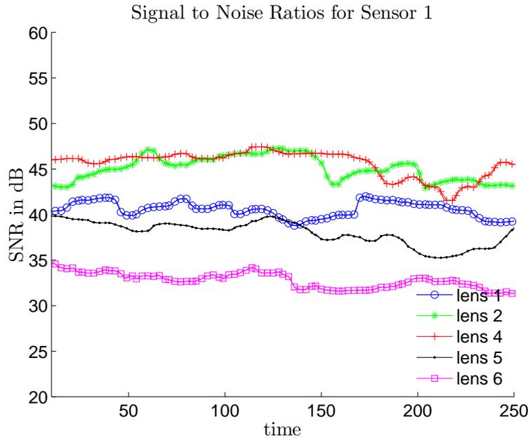
Figure 8. SNR results of sensor 1 for different lenses (250 consecutive measurements at 15fps, lens 3 omitted)
