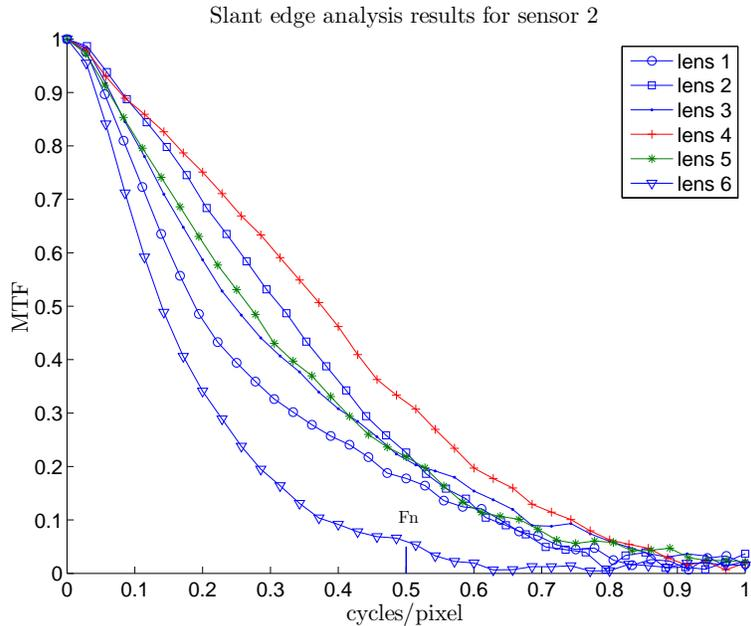
Figure 4. Normalized MTF for sensor 2 over cycles per pixel ( $F_n =$  Nyquist Frequency). Lens 4 shows the best performance, while the low performance of lens 6 even limits the sensors performance.
