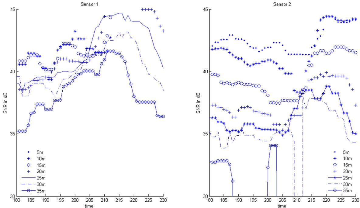
Figure 13. SNR evaluation for different distance segments of the scene shown in Fig. 12. Sensor 1 with lens 5 outperforms sensor 2 with lens 6 in distances above 25m but with the loss of information for road features under 10m due to the different perspective. The constant good quality of the markings is visible in the stepwise decreasing ratio from 5m on in sensor 2.
