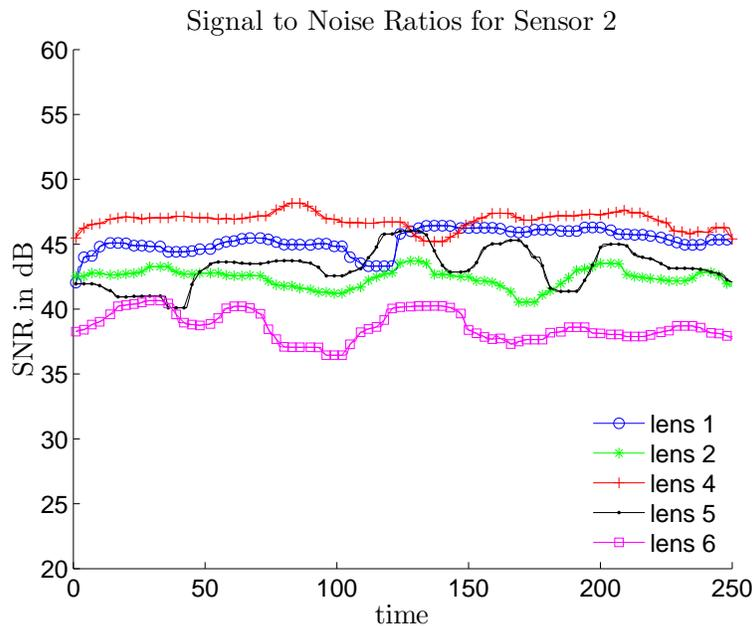
Figure 9. SNR results of sensor 2 for different lenses (250 consecutive measurements at 15fps, lens 3 omitted)
