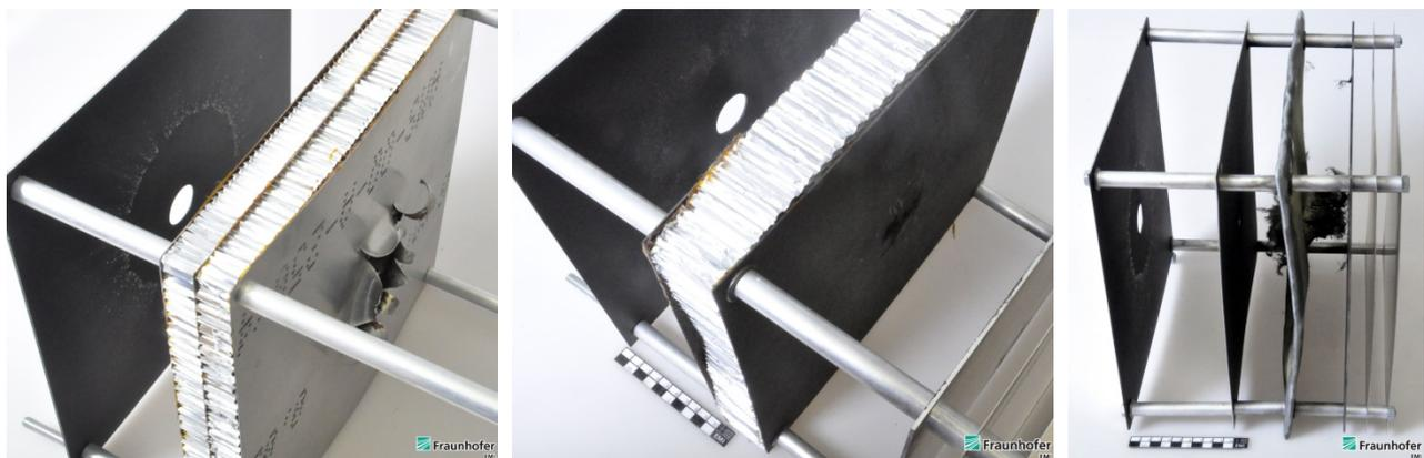
Figure 7. Example targets after impact testing. From left to right: aluminum sandwich panel (Target 2.3, experiment 5387), CFRP sandwich panel (Target 3.2, experiment 5404), intermediate layer or reinforced box wall (Target 5.2, experiment 5392).
