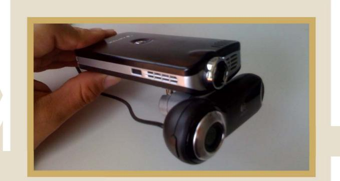
**Assembling** of a projector-camera system creates a mobile augmented interface to annotate physical media.
