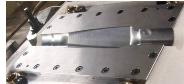
shell with die shape (front side)
