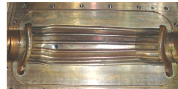
basic body with cooling channels
