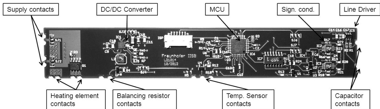
*Fig. 7: Smart battery electronics with microcontroller, signal conditioning and line driver, switches for the balancing resistor and heating element*
