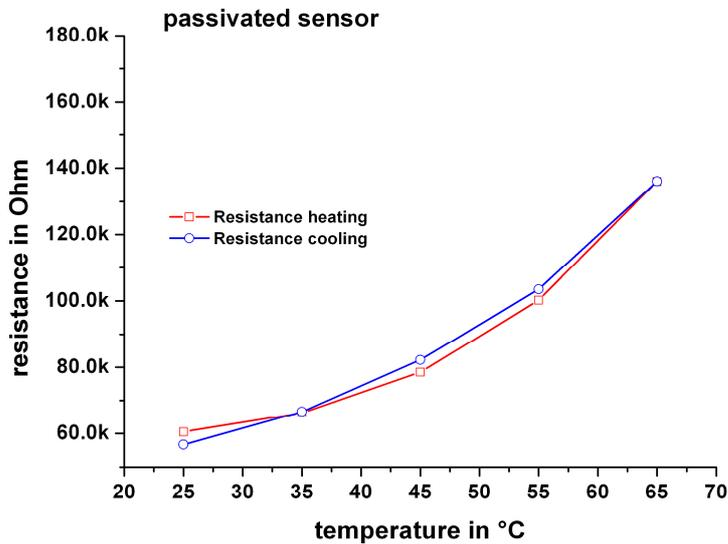
Figure 7: Thermal characterization of the carbon compound sample. The square (red) and round (blue) points show the averaged resistance values for both, heating and cooling phase. The two pictures show the hysteresis of the same temperature sensor without passivation layer (top) and with passivation layer (bottom).
