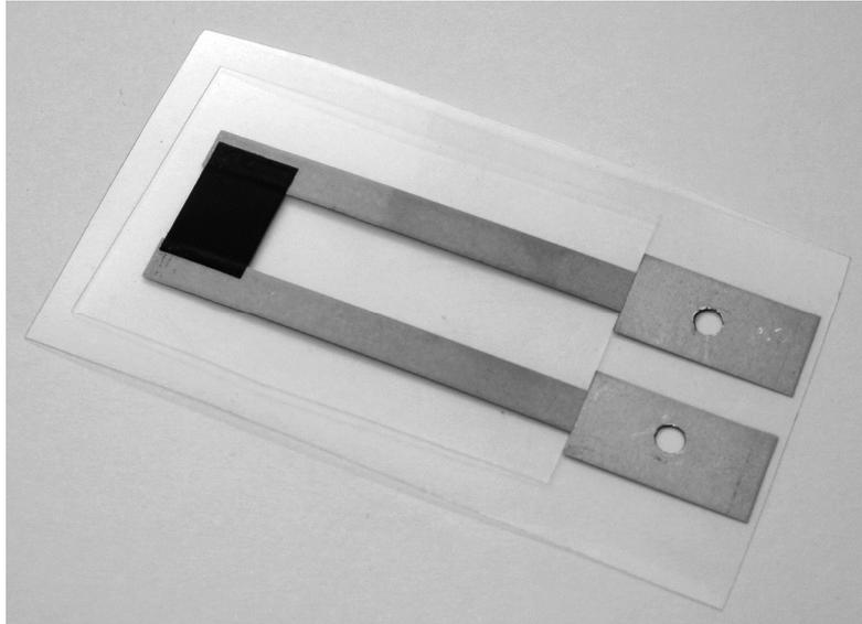
*Fig. 5: Printed temperature sensor on PE substrate.*
