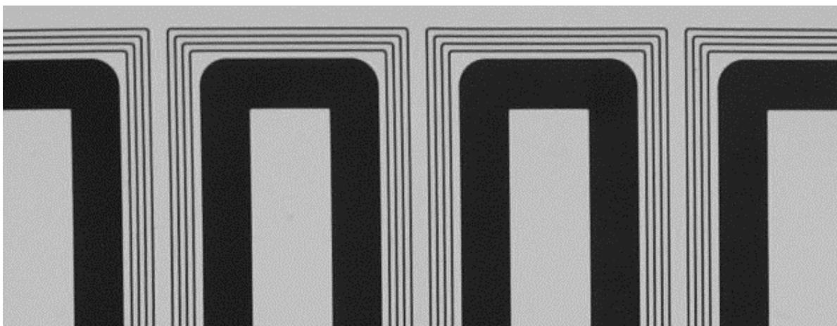
*Fig. 2: Detail of the heating element and balancing resistor structure.*
