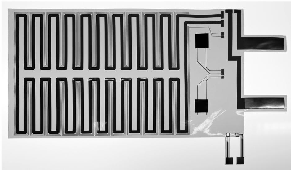
*Fig. 1: Flexible foil with integrated temperature sensor, balancing resistor and heating element.*
