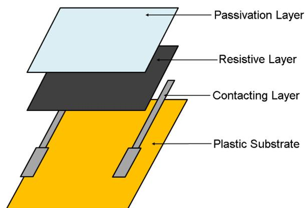
*Fig. 6: Design of the temperature sensor showing the stacked functional layers*
