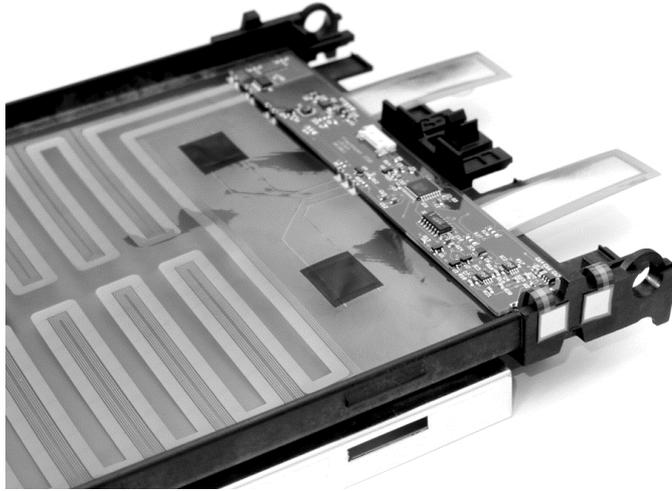
*Fig. 8: Flexible foil with smart battery electronics mounted on battery frame.*
