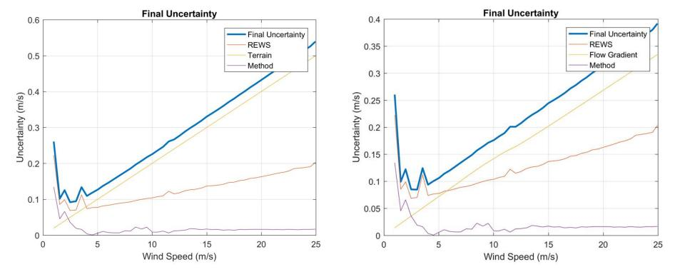
Although the RSD wind speed uncertainty is significantly reduced, this has no impact on the REWS (or final) uncertainty as the conventional wind speed uncertainty dominates (in this case). The reduction in final uncertainty is again down to the terrain/flow gradient uncertainty.
