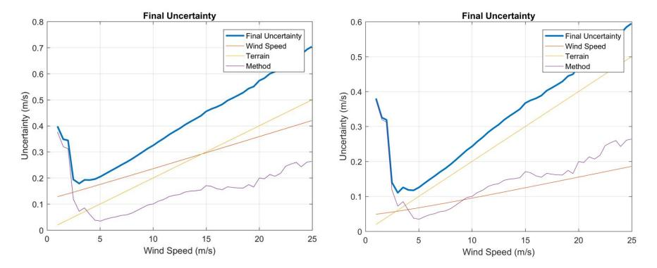
Correcting for the typographical error (in using the anemometer class number) reduces the classification error by a factor of 3. This in turn reduces the measured wind speed uncertainty and hence the final uncertainty.
