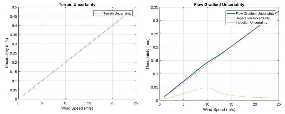
Assuming a typical flow gradient of 4%/km rather than applying a fixed 2% uncertainty has some benefit. (This is much more pronounced for offshore cases where the 0.05%/km may be assumed.)
