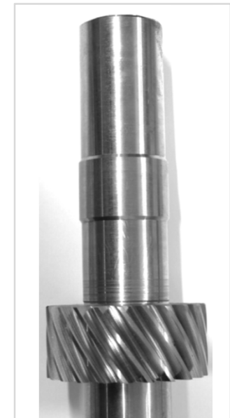
Demonstrator with rolled toothings
