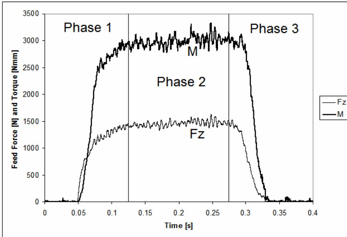
**Figure 1:** Phases of a drilling operation (5 mm drill diameter)
