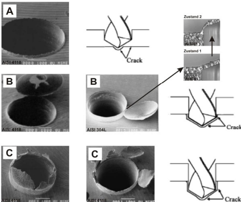
**Figure 3:** Drilling burr types [3], [4]
