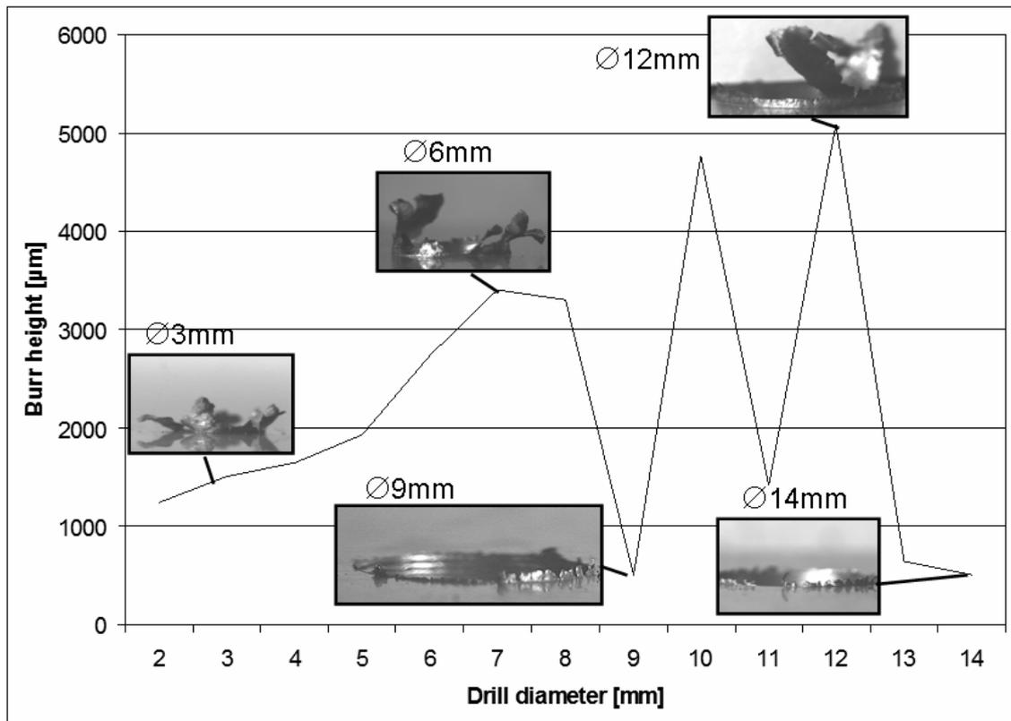
**Figure 6:** Comparison of the average burr heights for selected drill diameters
