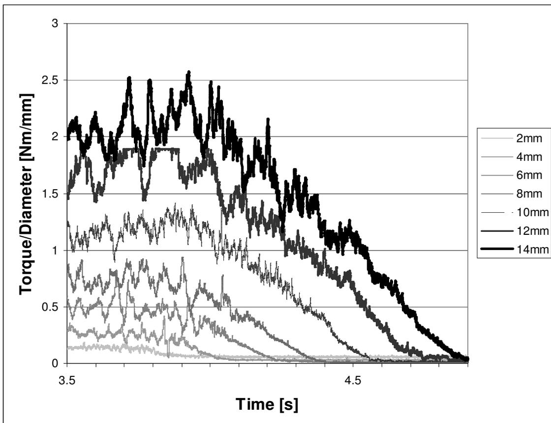
Figure 5: Torque during the burr formation
