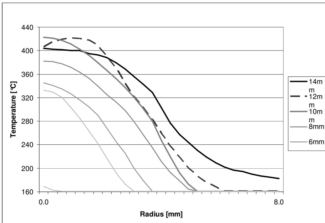
**Figure 7:** Temperature path over the radius before drill exit
