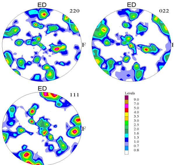
Figure 2. Pole figures of the hot extruded sample after post heat treatments (5% compressive strain and annealing under load) measured with HESR (ED - extrusion direction, F - compression direction)
