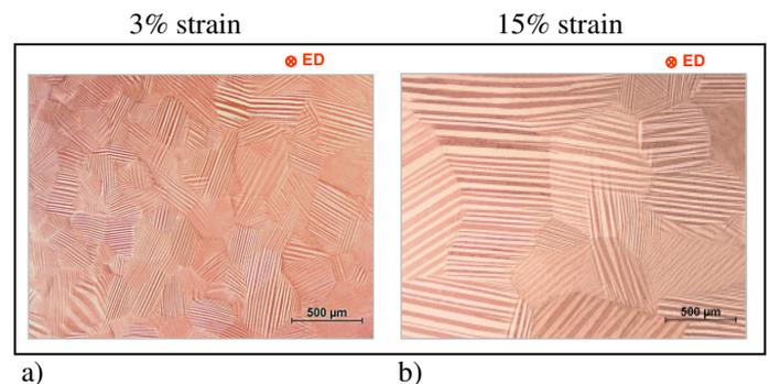
Figure 1. Microstructure of a hot extruded  $\text{Ni}_{50}\text{Mn}_{29}\text{Ga}_{21}$  alloy after different compressive strains and annealing under load (compression direction perpendicular to ED).
