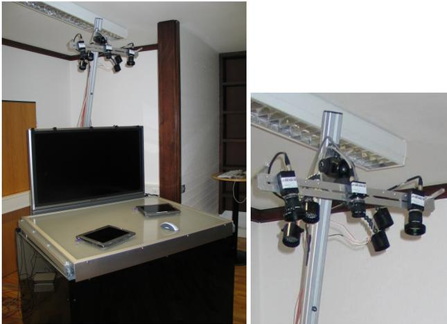
Fig. 3. Left: horizontal large display surface (gray) and two little displays (black) with high resolution lying upon the large display, vertical display for additional information (black), cameras 1.6 meters above the tabletop. Right: detailed view of cameras and illumination
