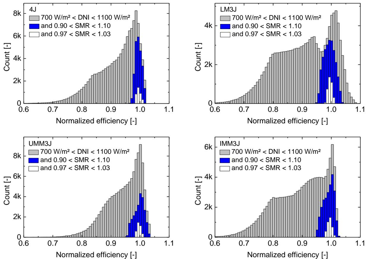
Figure 4: Efficiency of a four-junction (4J), lattice-matched (LM3J), upright metamorphic (UMM3J) and inverted metamorphic (IMM3J) triple-junction solar cell. The efficiencies are shown with filtering for DNI and additionally with SMR filtering using a Black Photon component cell sensor. The SMR filtering is done for SMR values within  $\pm 3\%$  and  $\pm 10\%$  of unity.
