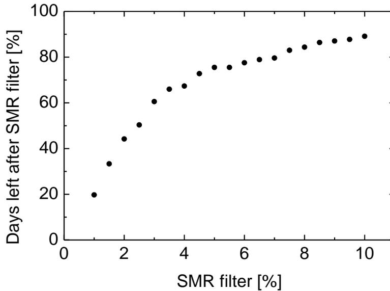
Figure 3: Percentage of sunny clear sky days left after SMR filtering. One year of data gathered at Fraunhofer ISE in Freiburg is used. For an SMR filter for  $SMR_{12}$ ,  $SMR_{13}$  and  $SMR_{23}$  of  $\pm 3.0\%$  around unity, 61 % of the measurement days are left. The measurement days left for power rating are nearly evenly spread over a period of nine months from February until October. The total number of clear sky days in 2014 in Freiburg was 147.
