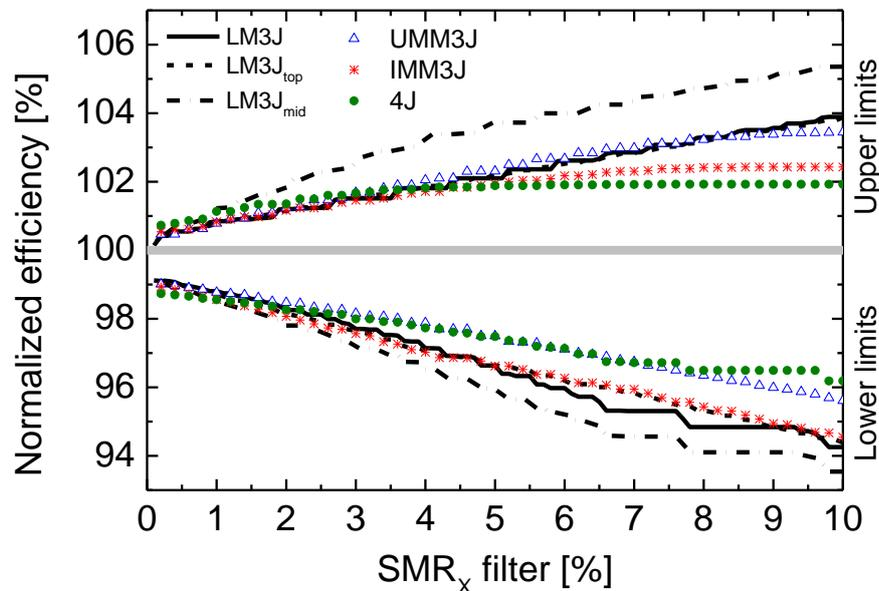
Figure 5: Upper and lower limit of the normalized efficiency of the investigated multi-junction solar cells as a function of SMR filtering. The efficiencies are normalized to the module efficiency at AM1.5d reference spectral conditions. The SMR values are calculated with the Black Photon lattice-matched components cells. The graph shows the upper and lower limits of the efficiencies left after SMR filtering. The same SMR filter percentage value is used for all three SMR values.
