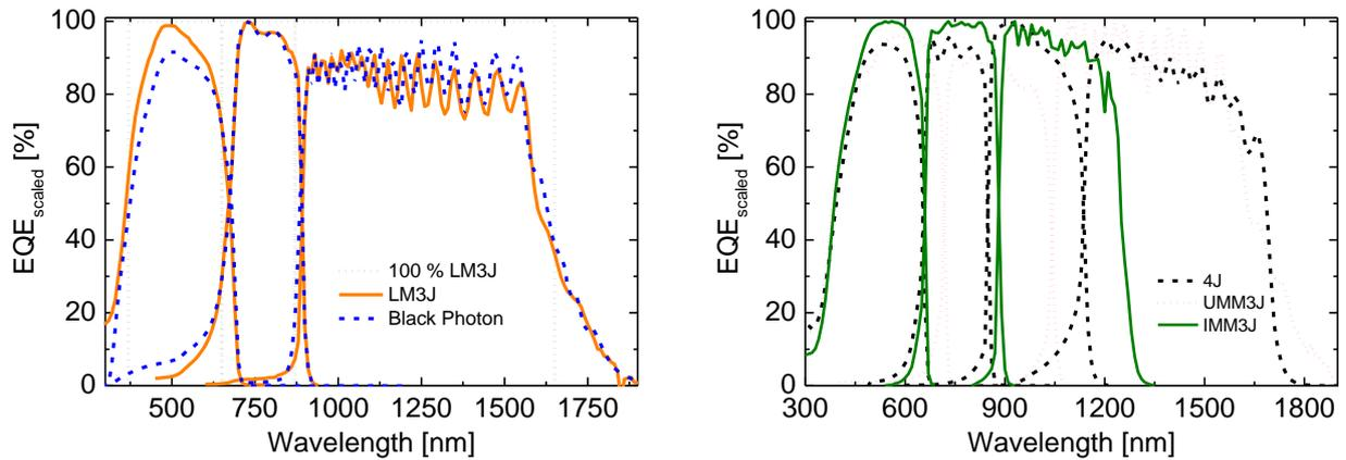
*Figure 2: External quantum efficiency (EQE) of the investigated cell concepts. The EQEs of all cell concepts are scaled in a manner that the sub cell with highest absolute EQE is normalized to 100 %. The same normalization factor is applied to the other sub cells, so that the relative difference between the sub cells is unchanged.*
