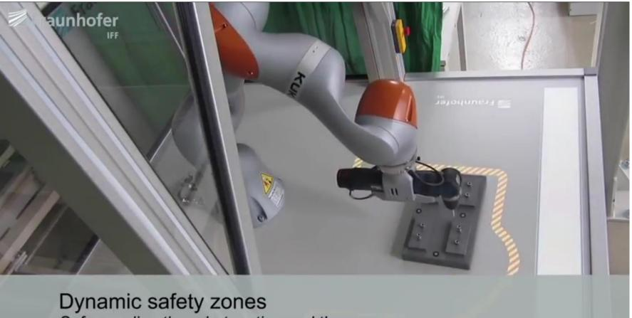
Safeguarding the robot motion and the process
