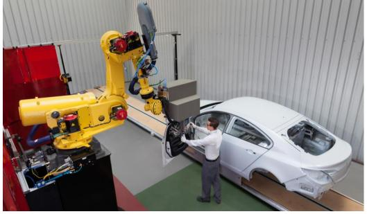
Exemplary application from Adam Opel AG for mounting door in final assembly area with HRC
