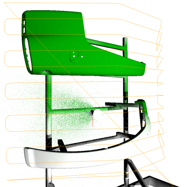
Fig. 9. A snapshot from the painting of the fender in IPS Virtual Paint.
