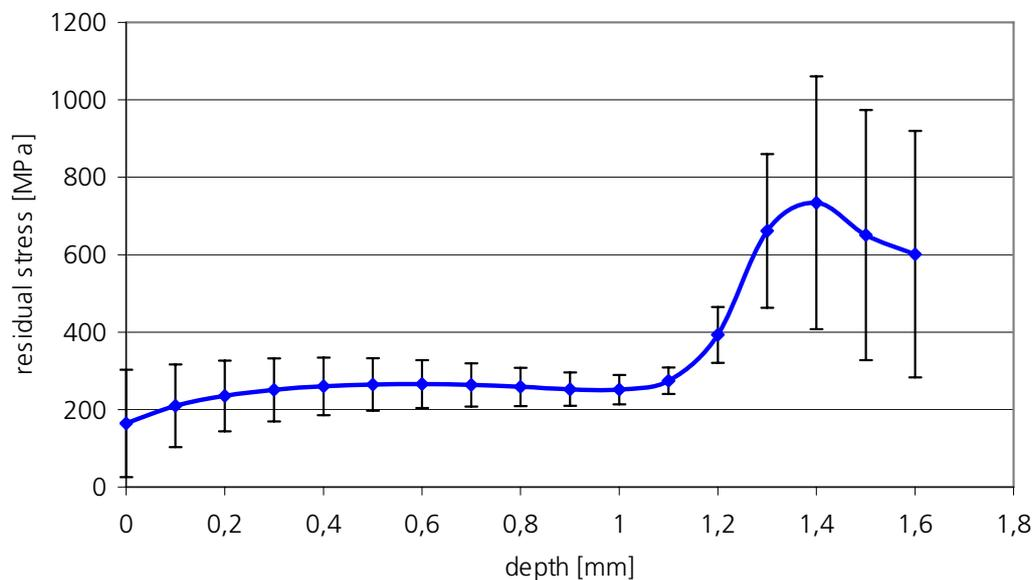
Figure 6: Mean stresses in direction of the tensile load stress (200 MPa) and appropriate standard deviations
