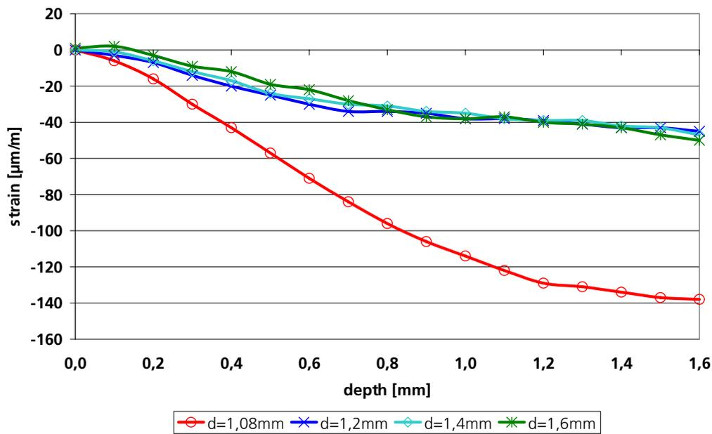
Figure 5: Measured strain development at the surface for increasing hole diameters (four cycles) in direction of the tensile load stress of 200 MPa
