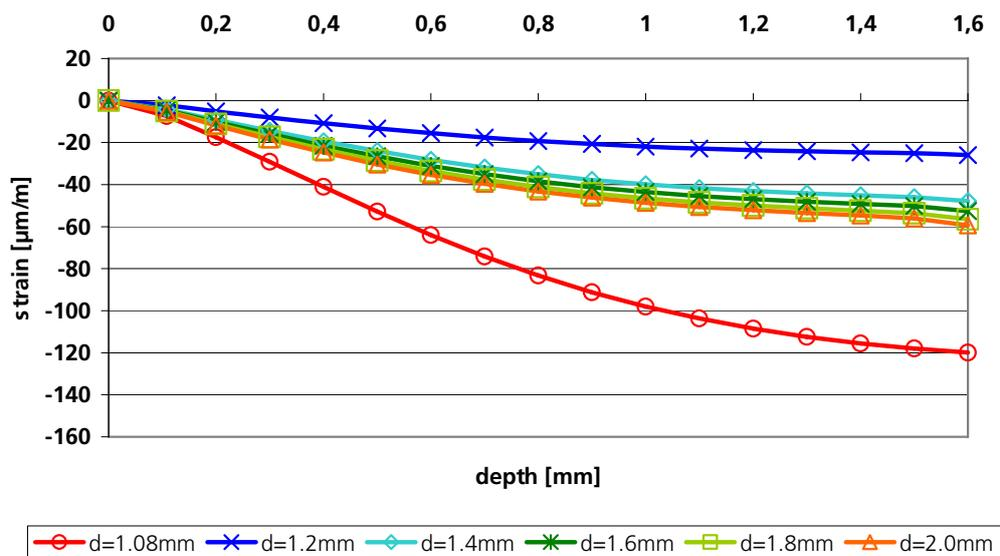
*Figure 4:* Numerically determined strain development (in loading direction) at the surface for increasing hole-diameters (tensile load stress of 200 MPa)
