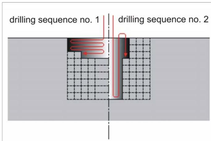
*Figure 1: Two possible drilling sequences with multiple stress relieves*
