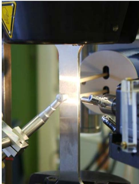
Figure 3: Hole drilling measurements on a test specimen under defined loading conditions
