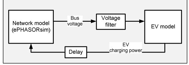
Fig. 7: Schematic diagram of simulation model
