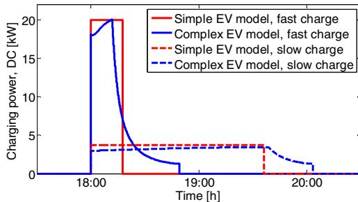
Fig. 4: Typical charging curves of different EV models and charging modes.
