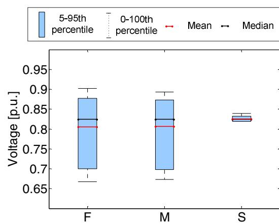
Fig. 5: Distribution of grid voltage minima by variation of EV charging positions with maximum EV penetration.
