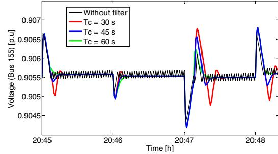
Fig. 8: Dynamic response of voltage with different filter parameter settings
