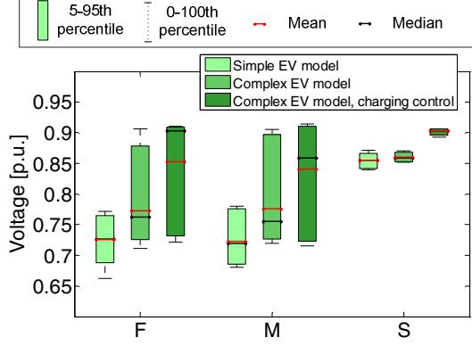
(b) Distribution of the lower bound 95th voltage percentile measured between 17:00 and 23:00.
