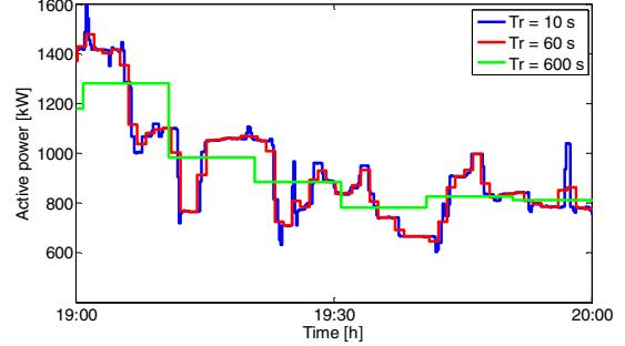
Fig. 1: Load profile (of one household) in different time resolutions.
