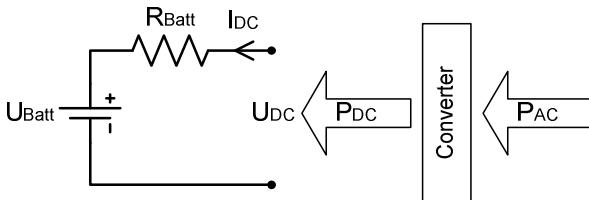
Fig. 2: Schematic diagram of the complex EV model.
