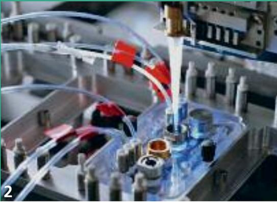
The holder plate offers space for ten Lab-on-a-Chip systems, several microtiter plates and a tip changing system, which consists of a magazine for one-way tips and measurement and ejection systems.
