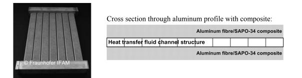
*Figure 5 – AdHex prototype and scheme of geometry with square fluid channels and fibre composite.*
