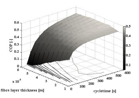
*Figure 8 - COP over fibre layer thickness and cycle durations: Results from parameter variation with bidisperse model, for parameters see Table 2.*
