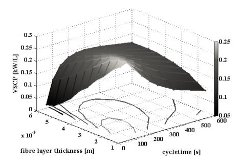
*Figure 7 - VSCP over fibre layer thickness and cycle durations: Results from parameter variation with bidisperse model, for parameters see Table 2.*
