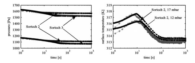
Figure 3 – Adsorption kinetics of the two pure adsorbent layer samples: measured pressure signals(grey) for both samples, two different starting pressures (left), for a better overview only surface temperatures of Sortech 2 for the two starting pressures (right). Simulated results for single layer samples Sortech 2 (o) and Sortech 3 ( $\diamond$ ) in black. Parameters for the simulation can be found in Tables 1 and 2.
