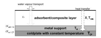
Figure 2 – Schematical presentation of a sample on the coldplate, heat transfer is influenced by the thermal conductivities of the adsorbent (composite) layer and the metal support as well as the two heat transfer coefficients between the layers.
