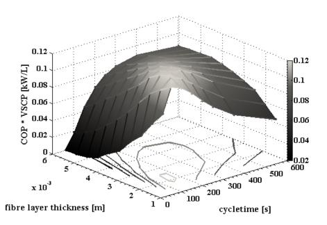
*Figure 6 - Product of COP and VSCP over fibre layer thickness and cycle durations: Results from parameter variation with bidisperse model, for parameters see Table 2.*
