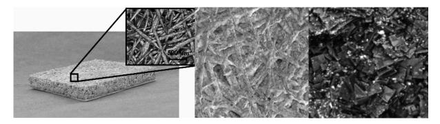
Figure 1 – Sample IFAM 1378: Fibres sintered to an aluminum sheet without adsorbent (left,full sample size  $30x30mm^2$ ), fibres with SAPO-34 deposition (middle, fibre thickness ~120µm), laser scanning microscope picture of SAPO-34 crystals on fibre (right, crystal size ~10-20µm).
