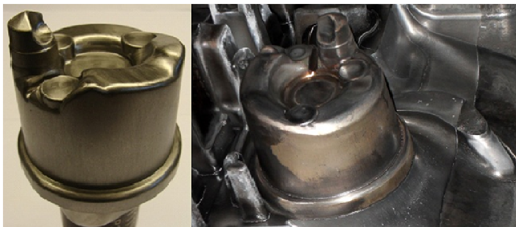
Figure 13 - laser beam melted tool insert (left) and installed as a component in the die (right)
