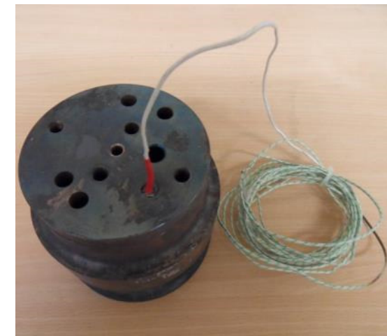
Tool insert with integrated thermocouple (type K)
