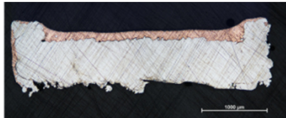
Multi-material sample Steel (LBM) with copper inlay (dispensing)
