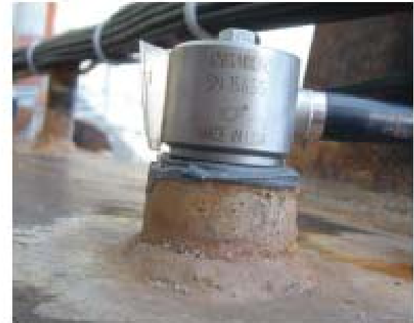
Acoustic sensor (acoustic emissions into the water)
