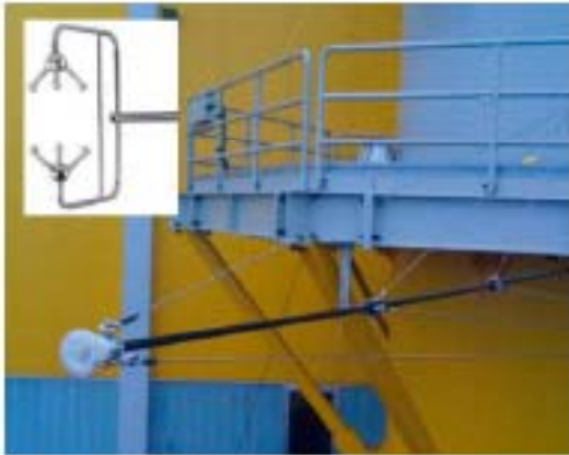
Carbonmast for high-resolution wind measurement
