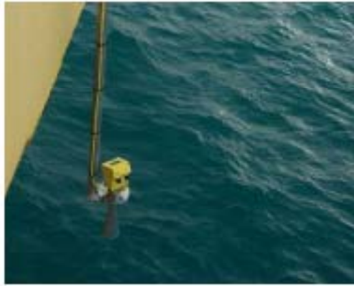
Radar for wave height measurement
