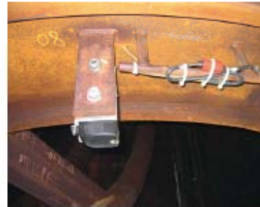
Sonars (sediment modification, scouring)
