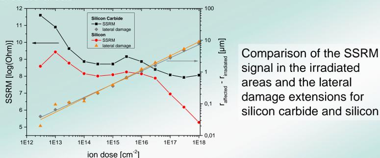
Comparison of the SSRM signal in the irradiated areas and the lateral damage extensions for silicon carbide and silicon
