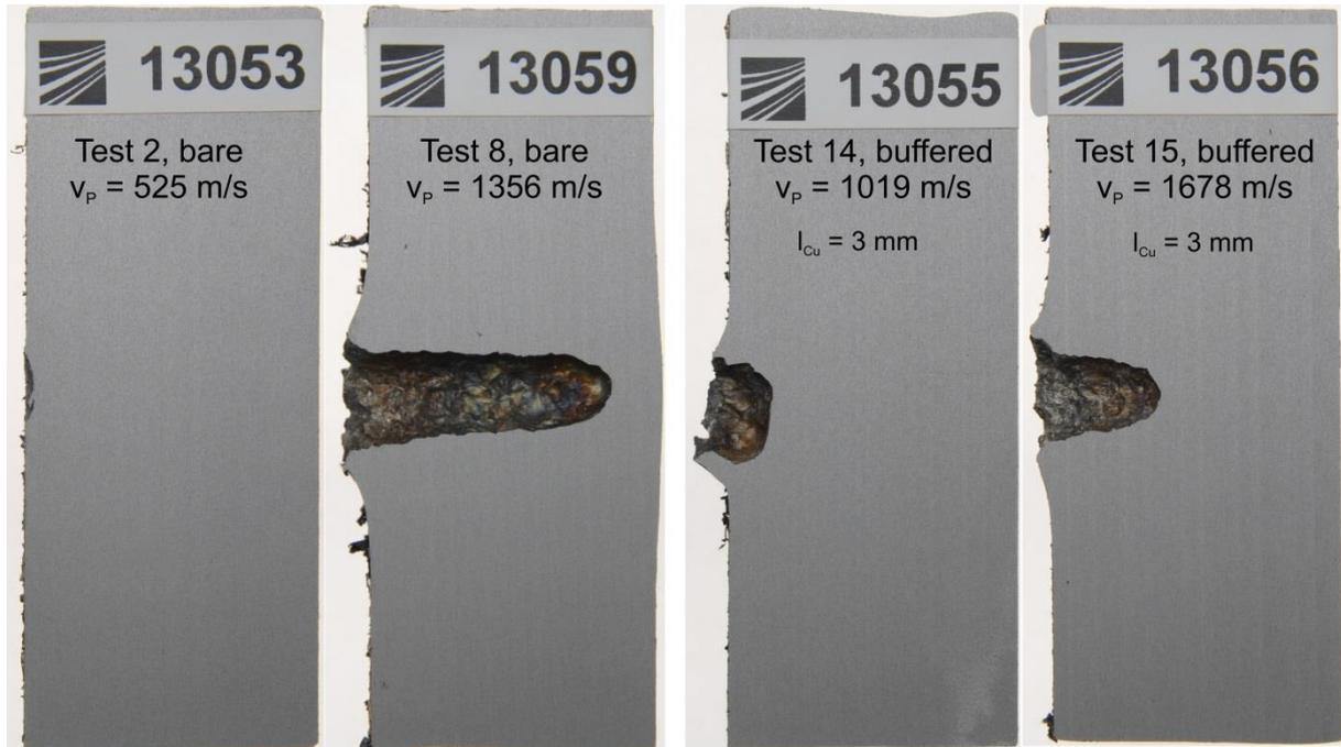
Figure 5: Crater images for the bare target (Tests 2 and 8) and the buffered target (Tests 14 and 15)
