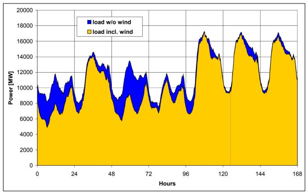
Figure 1: Load profile of E.ON Netz in 05/2003 including wind generation
