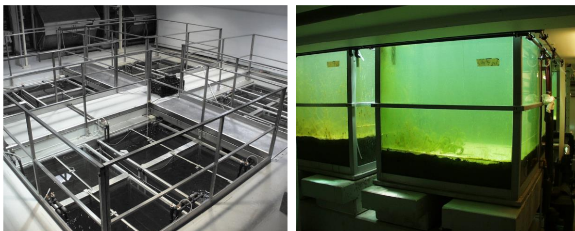
Figure 18: Indoor microcosm facility for focused community level and extended laboratory studies Water and sediment from natural sources; Volume 16 * 1 m 3 ; controlled temperature and light regimen (25 000 lx, sunlight spectrum); application of radio-labeled test substances possible
