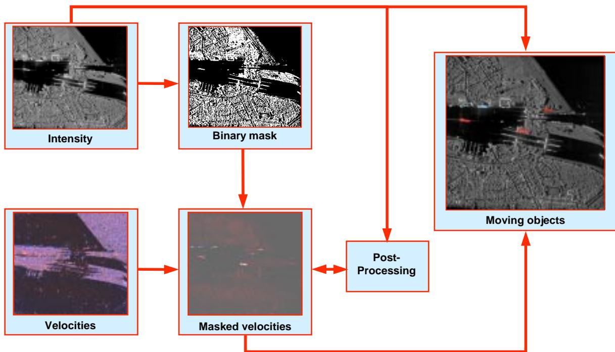
**Figure 1:** Workflow for the segmentation of moving objects in along-track interferometry data
