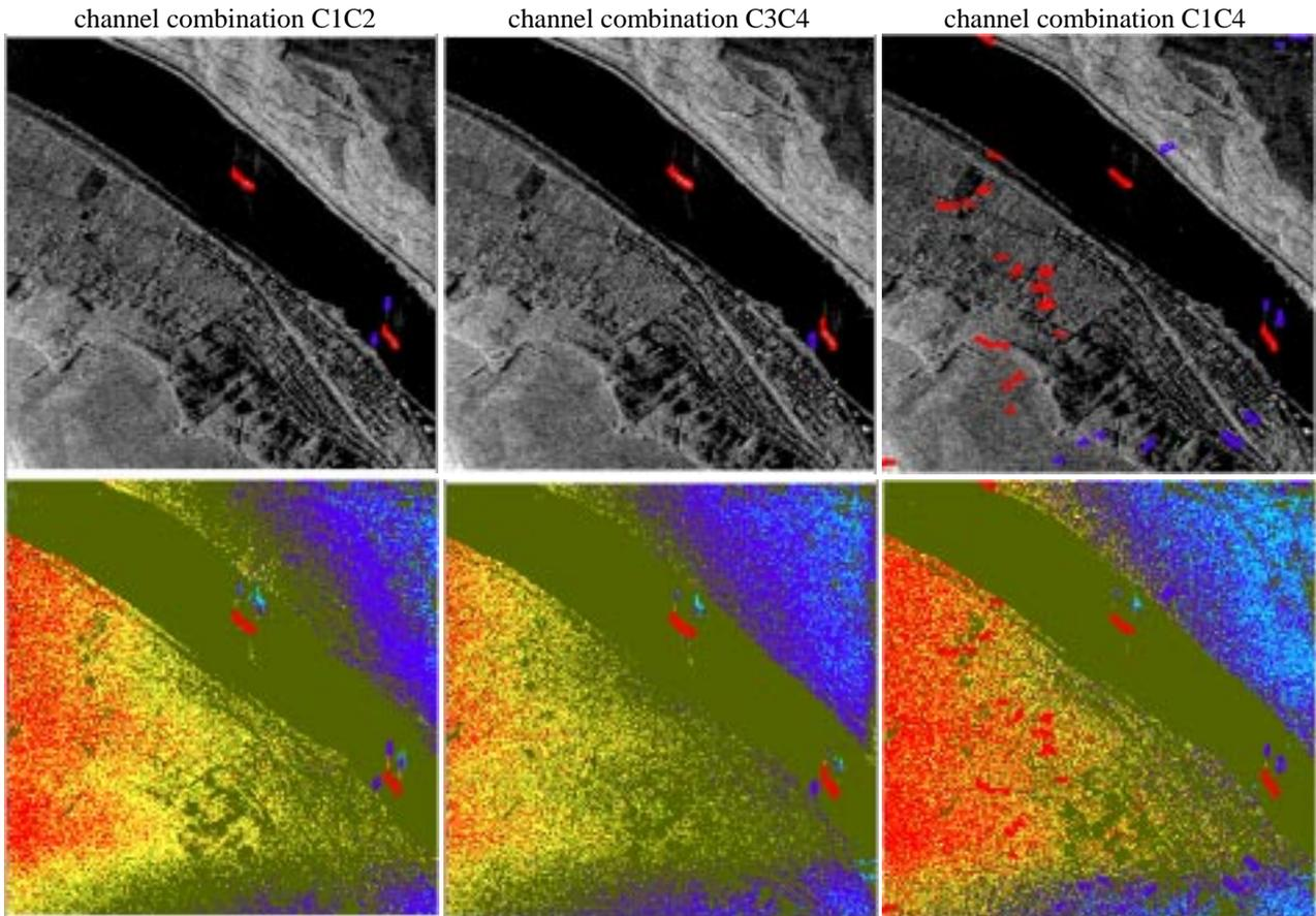
**Figure 2:** The upper row shows the segmentation result for different channel combinations as overlay on the intensity image and the lower row shows the corresponding phase differences (pseudo color scheme)
