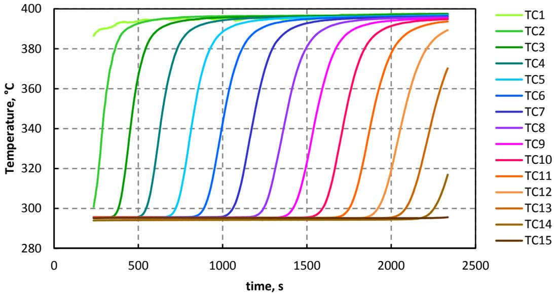
FIGURE 5. Temperature as function of the time for the different sensor positions (TC1 = top, TC15 = bottom).
