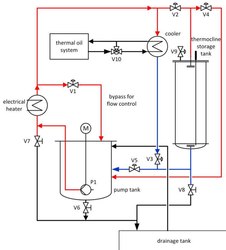
**FIGURE 1.** Layout of the single-tank test facility.
