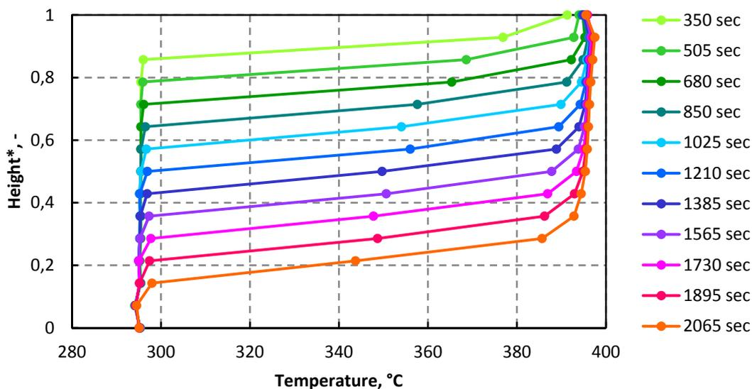
FIGURE 4. Stratification profile during a charging process with a small temperature difference.
