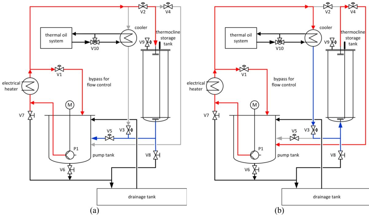
FIGURE 2. Illustration of the charging (a) and discharging process (b).
