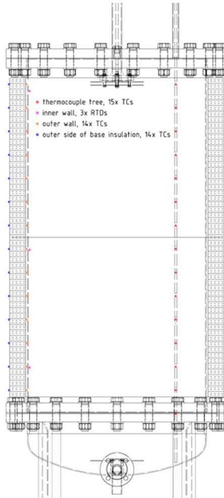
**FIGURE 3.** Instrumentation of the thermocline storage tank.
